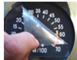
Once the transfer is removed, you will have a completely restored gauge face. The markings have a strong adhesive and will stay in place. For added security an **optional** light coat of satin clear may be applied over the entire face. Krylon makes a UV resistant satin clear that is excellent.
