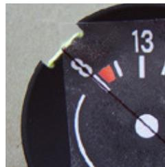
**Step 4** – Peel the clear transfer sheet from the gauge as described in section 6. The gauge face is now restored.
