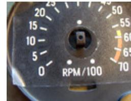
**6. Removing the Transfer** – The clear transfer sheet is removed from the gauge face in the same manner as it was removed from the white backing. Start at one corner and remove slowly, once again making sure that the markings have adhered to the gauge face.
